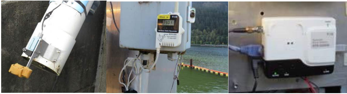
Figure 3. Mechanical counter components used to enumerate lamprey passage including the limit switch attached to exit paddle and cushion, wireless data recorder, and network base station (from left to right).
